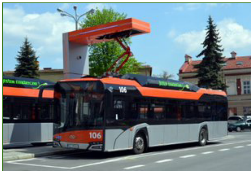
Photo 23. Electric bus - fast charging. Source: City Hall in Rzeszów
